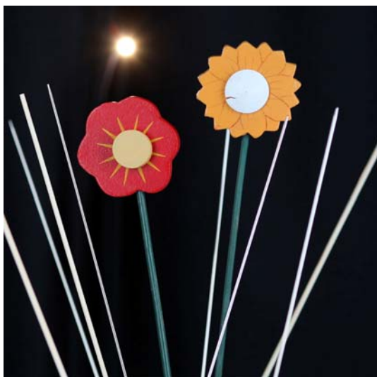
Test subject: two flowers which are not wilting under a spot-light, slivers of wood and metal knitting needles as a model for blades of grass and, in the background, a small, bright, circular light source as an iris indicator.
